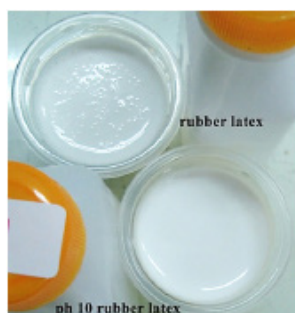
Figure 3 Textures after pasteurization of rubber latex and rubber latex adjusted to pH 10
