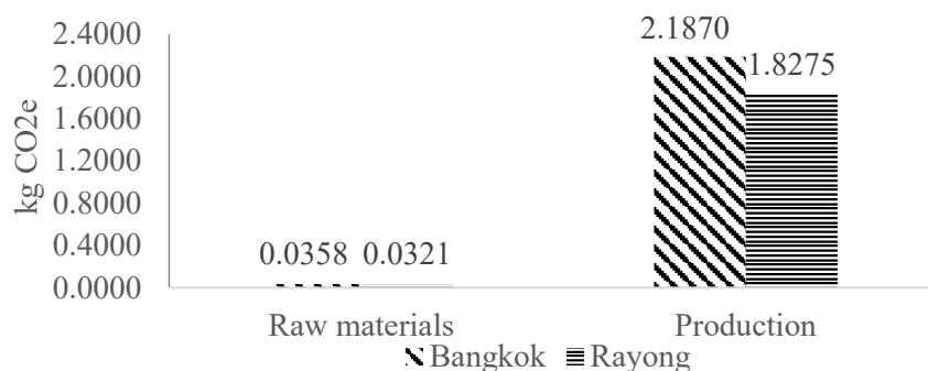
Figure 4. GHG of Post-Consumer PET bottle raw materials and production (Factor unit: 1 kg used PET bottles) of Bangkok and Rayong province
