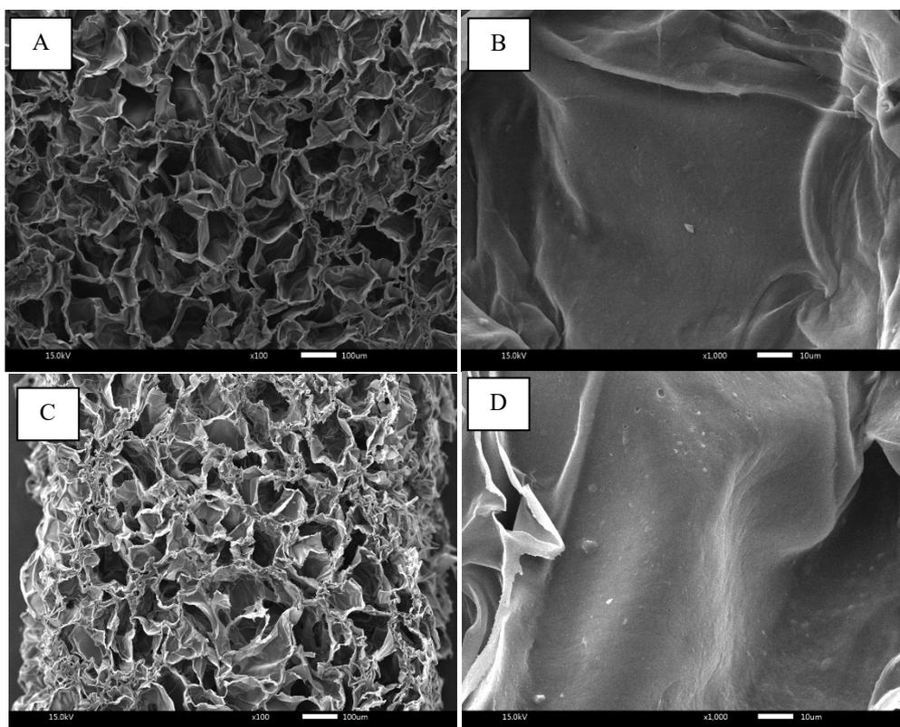
**Figure 1.** SEM-EDS micrographs of scaffolds after freeze-drying, methanol treatment, and autoclaved; (A) 2%SF/1%C, (B) 2%SF/2%C at a magnification of 100X; (C) 2%SF/1%C, (D) 2%SF/2%C at a magnification of 1000X. Scale bar = 100  $\mu$ m.
