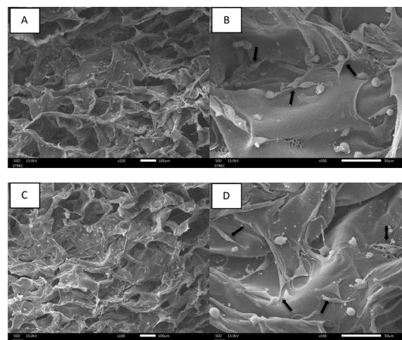
**Figure 3.** SEM-EDS micrographs of scaffolds cultured with HEC-2 cells for 7 days; (A) 2%SF/1%C, (C) 2%SF/2%C at a magnification of 100X; (B) 2%SF/1%C, (D) 2%SF/2%C at a magnification of 500X. Black arrows indicate human corneal epithelial cells.
