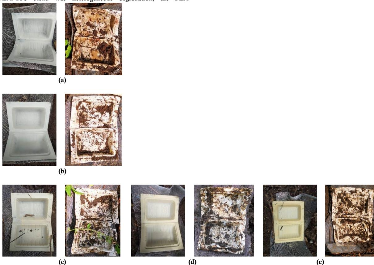
**Figure 1.** Appearances before (left) and after (right) soil burial biodegradation of (a) PLAPLA/TPS and (b)-(e) PLA/TPS/black pepper encapsulation; (b) PLA/TPS/BP-HPBCD10, (c) PLA/TPS/BP-MG10, (d) PLA/TPS/BP-MG15, and (e) PLA/TPS/BP-MG20.
