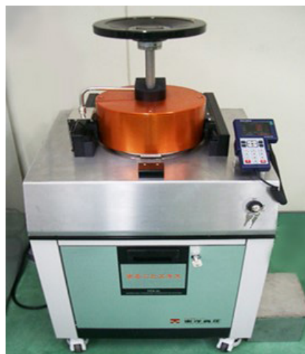
Fig. 1 High pressure processing apparatus (Toyo Koatsu Inc.)
