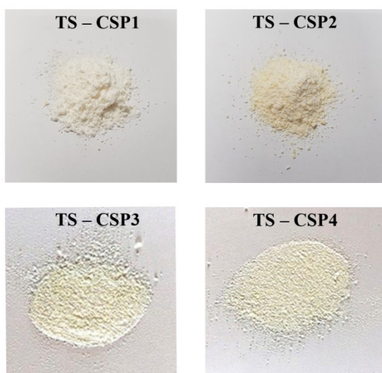
Figure 2. Appearances of TS-CSP hybrid materials prepared with different starch: chitosan ratio.
